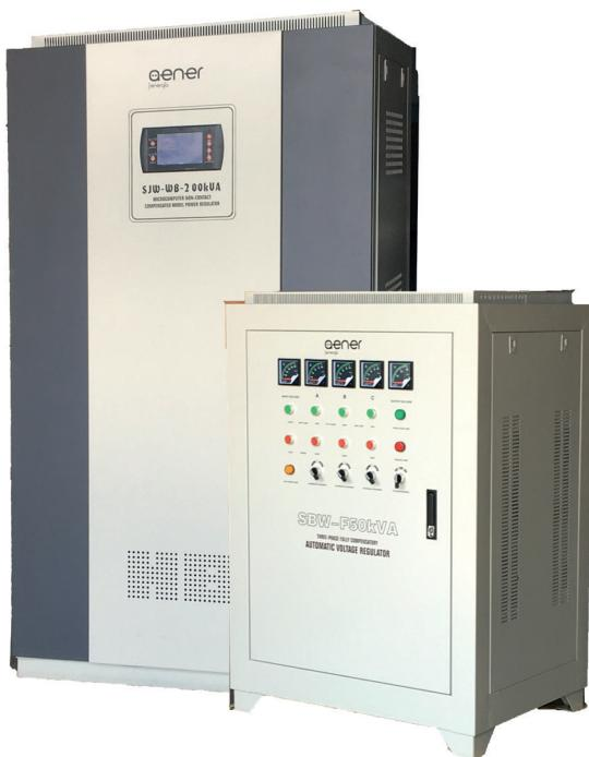
SBW Series Power Stabilizer is high accuracy fully automatic AC equipment. It consists of auto-transformer, servo motor, electronic control circuit and protections, besides measurement elements.
